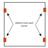
All fixings, where possible, should go into steel reinforcing.
